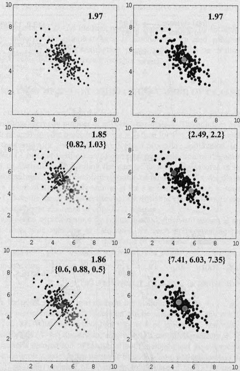
Figure 2. Comparison of effects of classification by *ISODATA* method (left column) and method of approximation by points (right column) for  $k = 1, 2$  and  $3$  – questionable example of classification
