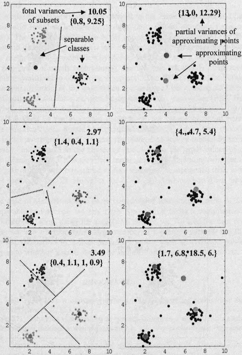
Figure 1. Comparison of effects of classification by *ISODATA* method (left column) and method of approximation by points (right column) for  $k=2, 3$  and  $4$
