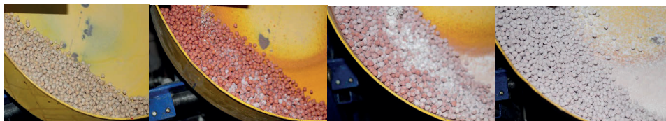
Figure 3.2.2. The process of pea seed coating on a disc granulator
