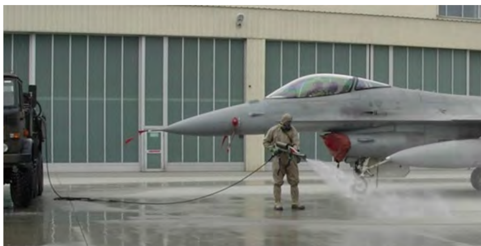
Figure 22. Decontamination process of an aircraft by SANIJET high-pressure washer as part of IRS-2C (author's photo)
