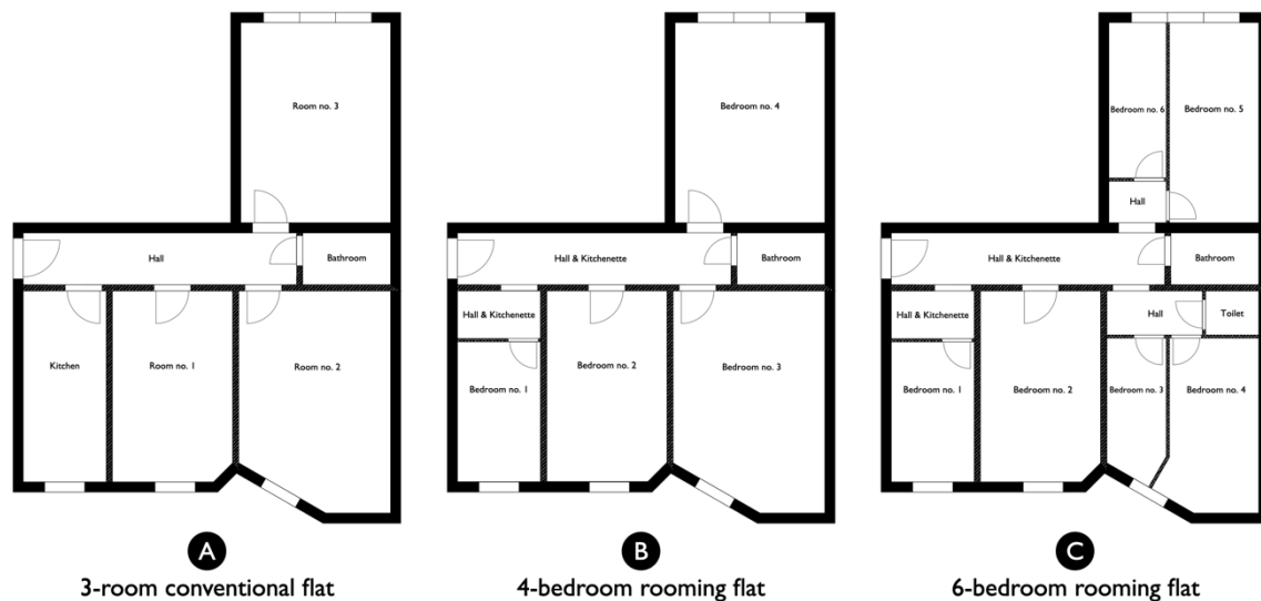
Figure 1. The layout of a conventional flat of ca. 75 square metres (A), its potential conversion to rooming flats following the ‘window-counting’ rule (B), and abandoning the rule (C).
