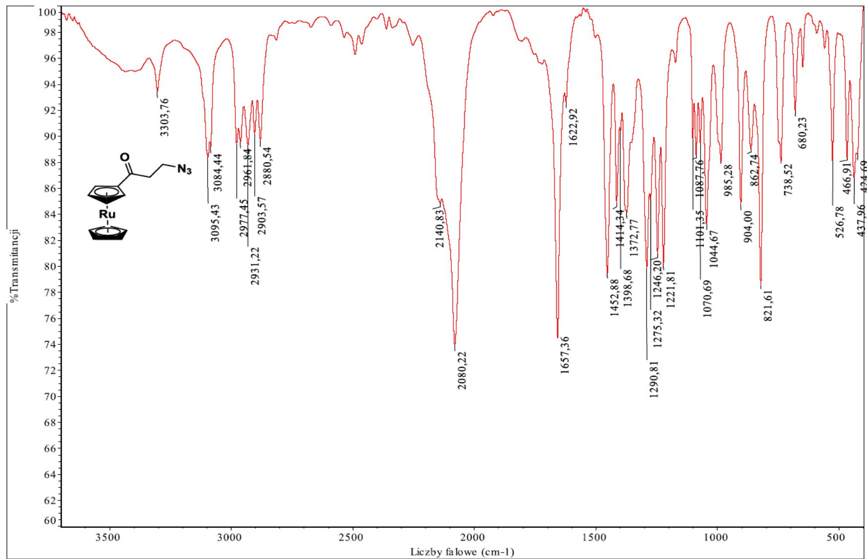
**Fig S40** FTIR (KBr  $\nu$  [cm<sup>-1</sup>]) spectrum of **2**
