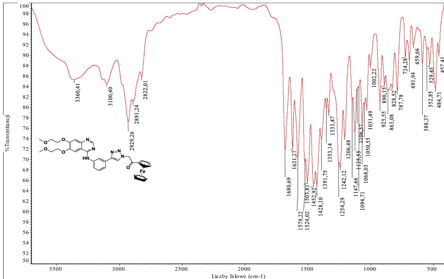
**Fig S41** FTIR (KBr  $\nu$  [ $\text{cm}^{-1}$ ]) spectrum of **3**
