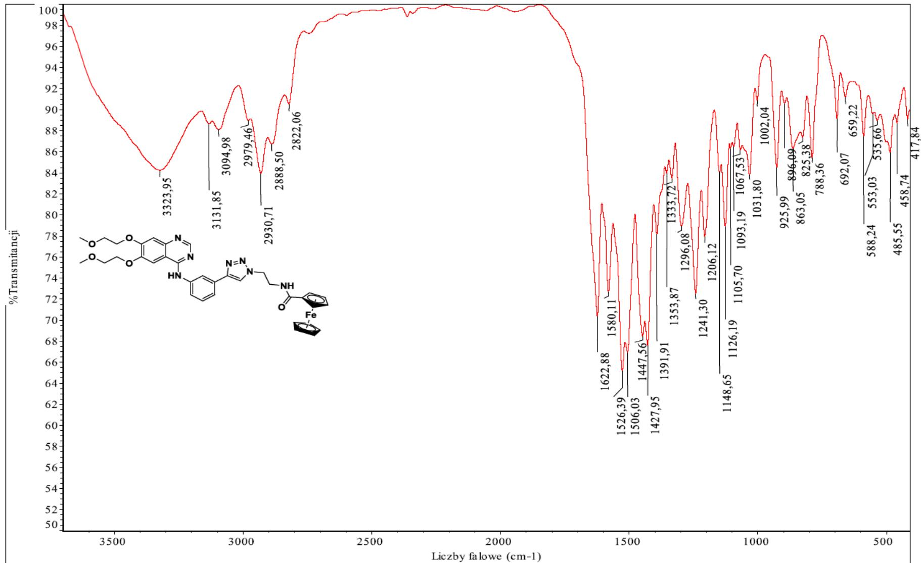
**Fig S46** FTIR (KBr  $\nu$  [cm<sup>-1</sup>]) spectrum of **8**
