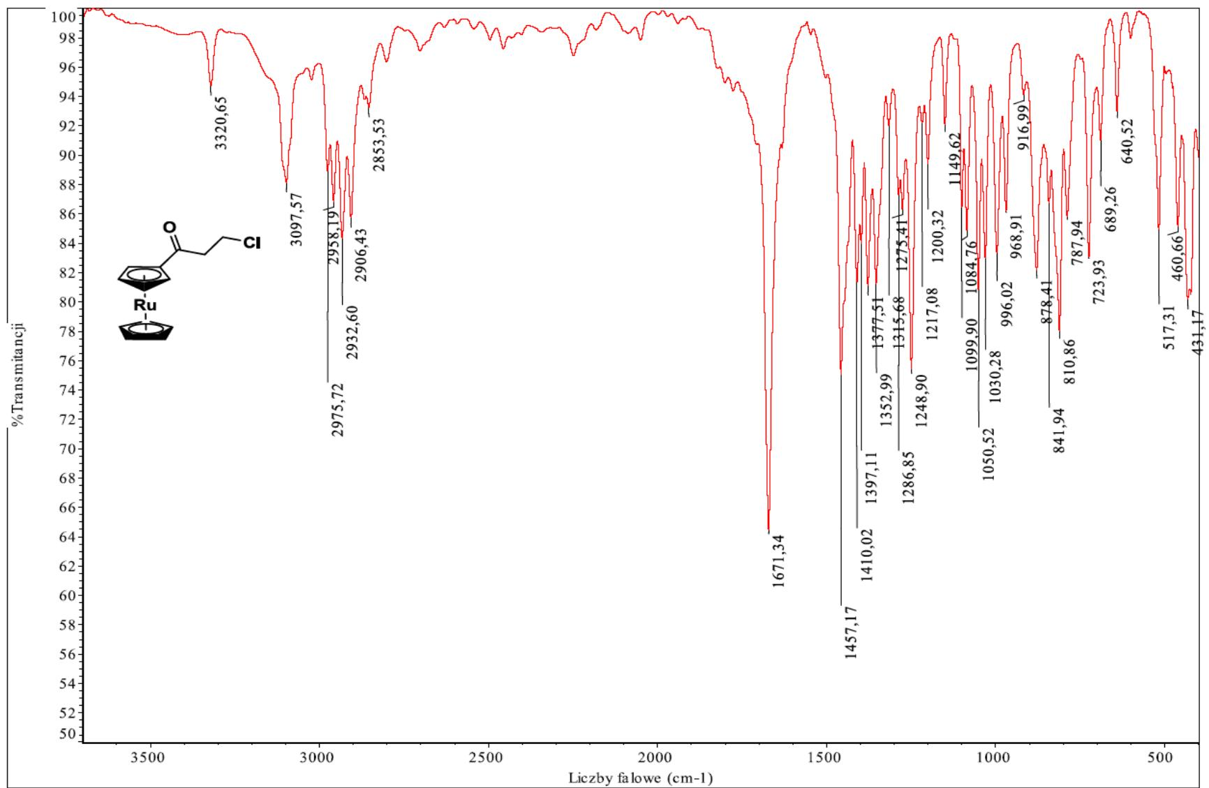
**Fig S39** FTIR (KBr  $\nu$  [cm<sup>-1</sup>]) spectrum of **1**
