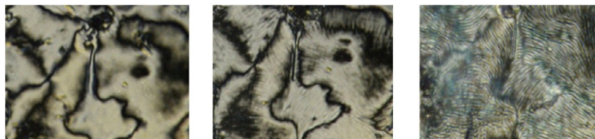
Fig. 10 The optical textures of 23a phases, respectively, from the left: SmC, B 1Rev , and B 1Rev' (2016JMCC11540). Reproduced by permission of The Royal Society of Chemistry.
