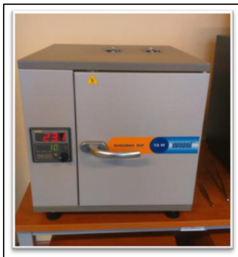
Fig. 6.6: Laboratory dryer SUP-18 W.
