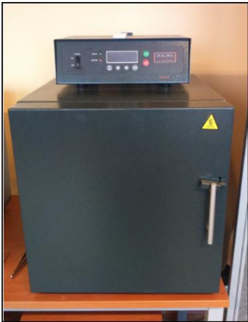
Fig. 6.4: Annealing furnace MT 1105-E4.
