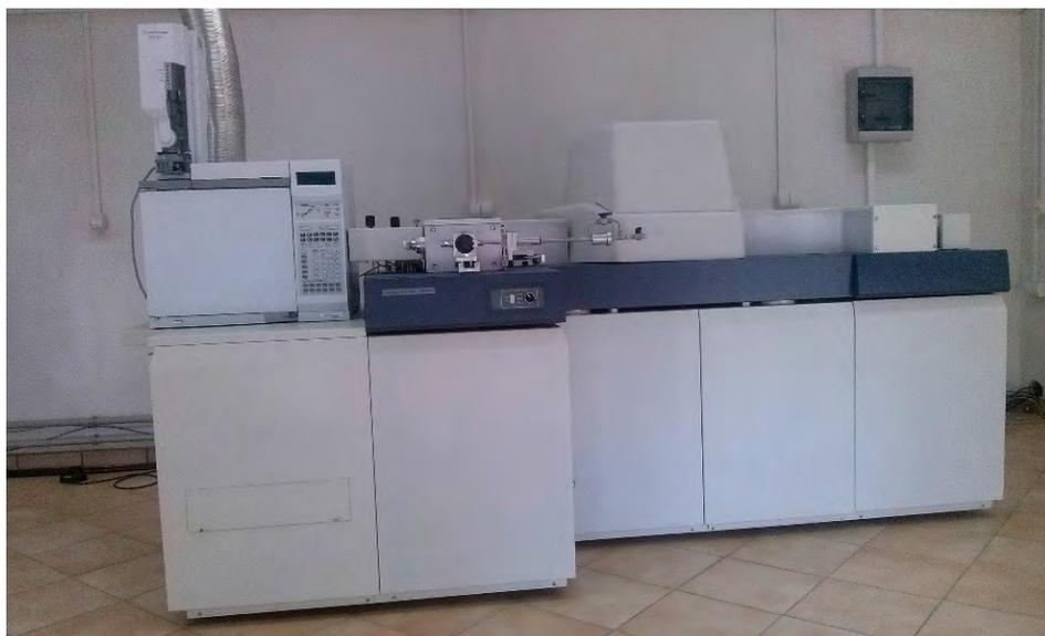
**Figure 29.** Micromass Autospec GC – HRMS (High Resolution Mass Spectrometer)
