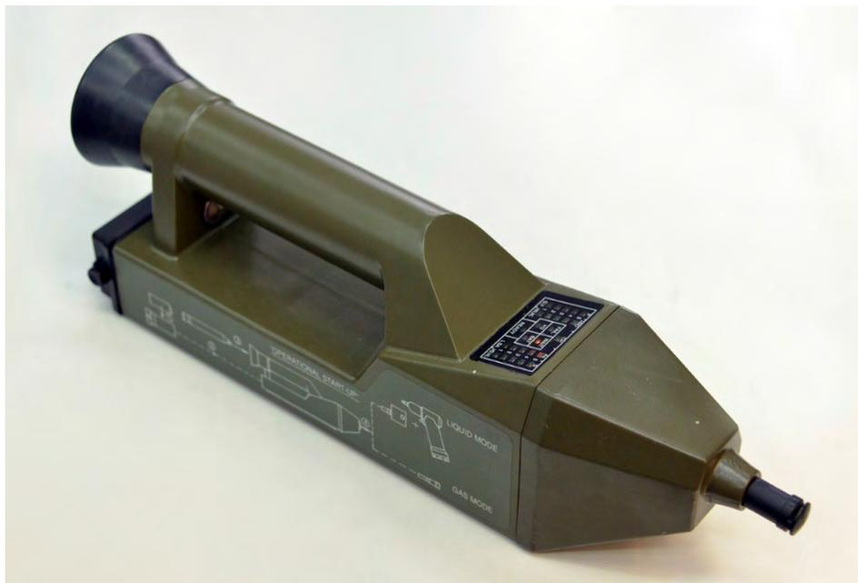
**Figure 16.** A Proengin AP4C FPD field detector, with an S4PE liquid sampler (author's photo)
