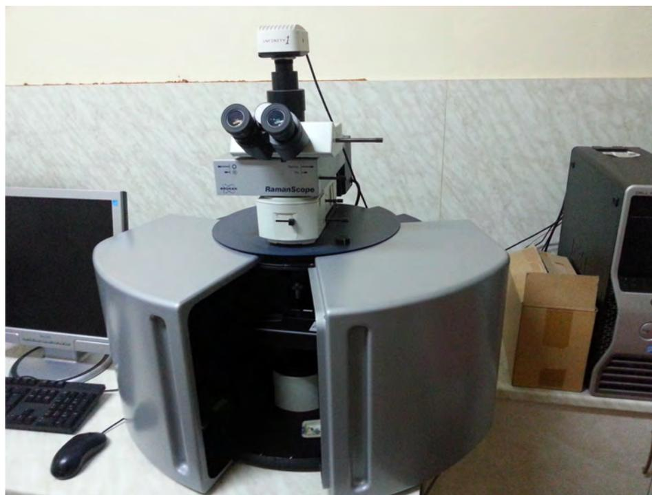
Figure 27. Bruker RamanScope III (author's photo)
