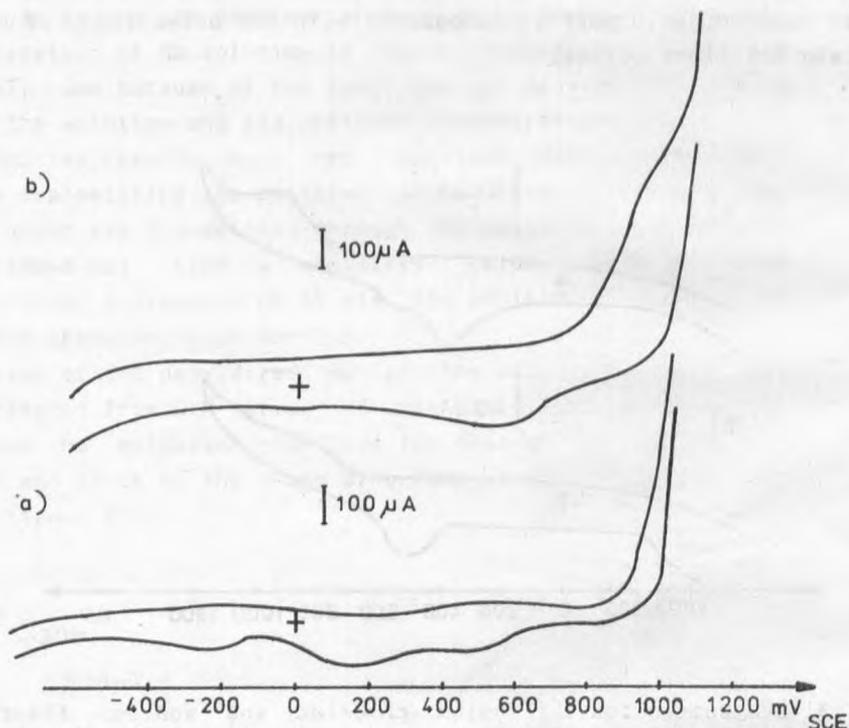
Fig. 4. CVM curves for the sodium chloride and sodium fluoride solution (0.5% NaF and 1% NaCl in voluminal ratio 1:100): a) not containing Hb; b) containing Hb. Sweep potential rate  $v = 0.05 \text{ V}\cdot\text{s}^{-1}$
