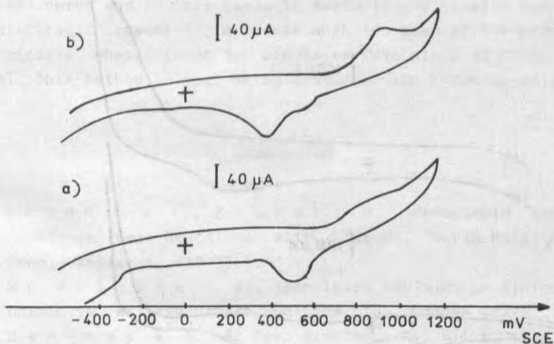
Fig. 3. CVM curves for the sodium chloride and sodium fluoride solution (0.5% NaF and 1% NaCl in voluminal ratio 100 : 1): a) not containing Hb; a) containing Hb. Sweep potential rate  $v = 0.02 \text{ V}\cdot\text{s}^{-1}$
