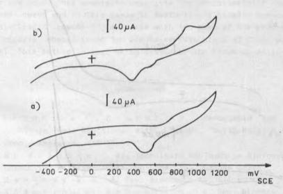
Fig. 3. CVM curves for the sodium chloride and sodium fluoride solution (0.5% NaF and 1% NaCl in voluminal ratio 100 : 1): a) not containing Hb; a) containing Hb. Sweep potential rate v = 0.02 V.s<sup>-1</sup>
